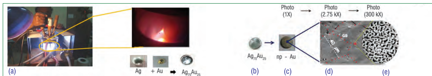
Figure: 1(a) Arc melting furnace set-up. (b), (c) Photographs of \text{Ag}_{75}\text{Au}_{25} alloy and nanoporous Au, respectively. (d), (e) SEM micrographs of nanoporous Au at two different magnifications
