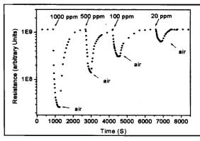
Fig. 4: Response characteristics of FeNbO, for different concentrations of H<sub>a</sub>
