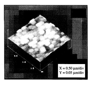
Fig. 3 : AFM micrograph of FeNbO<sub>2</sub> film
