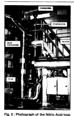
ultrasonic methods, and the ISI will be continued during maintenance shut downs to study the health of the loop components.
