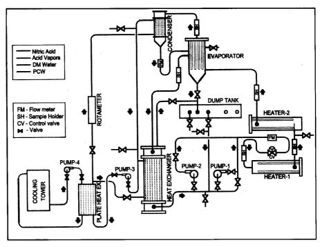
Fig. 1: Schematic flow diagram of the nitric acid loop
