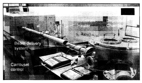
Fig. 2: Pulsed Laser deposition Facility
