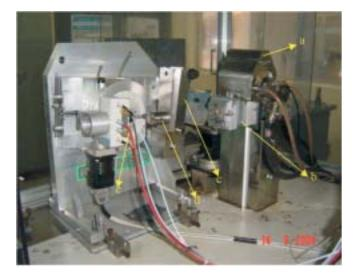
Fig. 2: Guiner Diffractometer setup. (a) 18 KW rotating anode X-ray generator, Mo target. (b) Crystal monochromator (c) Pressure cell holder (d) Diamond anvil cell (e) Position sensitive detector
