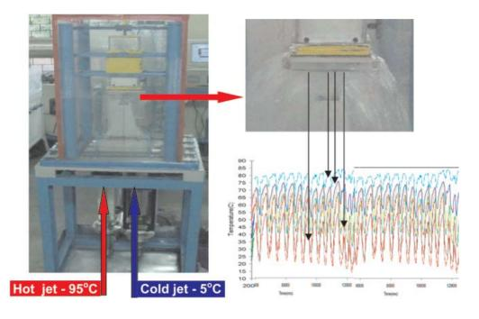
Fig.9 Simulation of thermal striping with water jets
