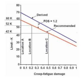
Fig.7 Thermal striping limits for PFBR
