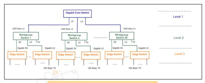
Figure 1: Upgraded Setup of Campus Backbone Network with Gigabit Technology
