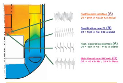
Fig.8: Thermal striping zones and temperature fluctuations in hot and cold pools of PFBR
