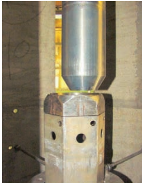
Figure 3: DSRDM & DSR with 30 mm Misalignment
