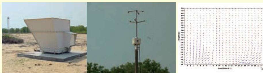
Figure 2: Boundary Layer Wind profiler and sonic anemometer used for diurnal wind and turbulence measurements at Thumba coastal site
