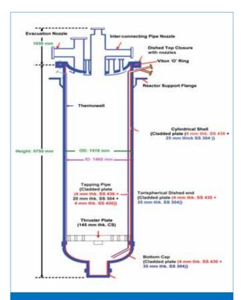
Figure1: Schematic of the Clad SS 304 / SS 430 Reactor (assembled) for KMML's 500 tonnes per annum titanium sponge
