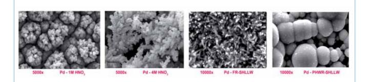
Figure 2: SEM images of palladium deposited from 1M and 4M nitric acid and Fast Reactor-Simulated High Level Liquid Waste and PHWR-Simulated High Level Liquid Waste solutions. Working electrode: stainless steel, counter electrode: platinum, quasi-reference electrode: Pd wire. T: 298 K. Duration of electrolysis: 8 hours. Applied cathodic potential: -0.5 V(Vs. Pd)
