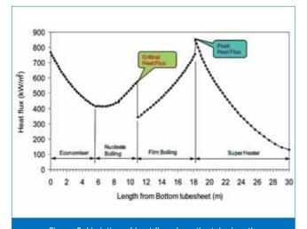
Figure 6: Variation of heat flux along the tube length
