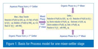
from the initial conditions to steady-state conditions and it provides important information about the variation of solute concentration with time in the contactor bank. Transient calculations can only provide the information about unsafe accumulation of solute if any. Simulation of almost all the published experimental results concerning to electrolytic partitioning of Pu/U were carried out in order to test the validity of the model equations and associated computer program.
