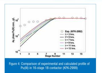
and Pu: 2.33 g/litre .The organic scrub is 20% in n-dodecane.The strip solution concentrations are:  $HNO_3$ :0.4M and  $N_2H_5^+$ :0.26M.The respective flow rates for feed, organic scrub and strip are 0.75, 0.156 and 0.12 litre per hour. The deviations in the plutonium profile in the low concentration are probably due to slow strip rate of Pu-HDBP complex and uncertainty in the estimation of distribution coefficient in low concentration region.
