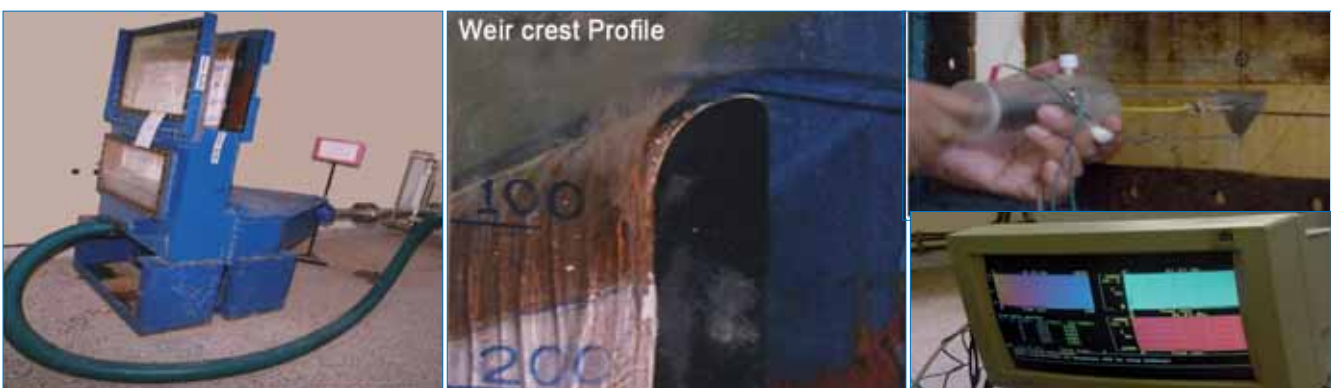
Figure 3: Weir – Crest testing full scale water model & water film thickness being measured by a special conductance probe connected to data acquisition system
