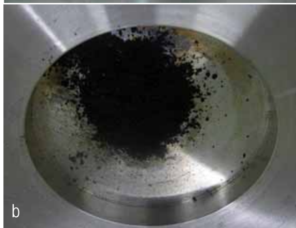
Figure 3: a) Small scale Sodium fire b) Sodium fire extinguished by carbon microsphere
