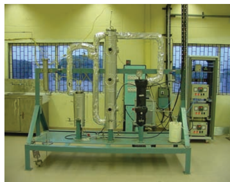
Figure 2: Pilot plant for sodium wetted component cleaning: water vapour - CO 2 process
