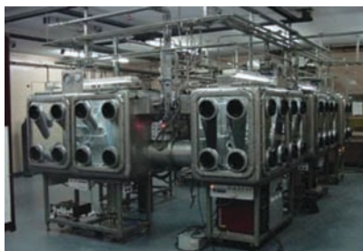
Figure 8: Glove box train facility for sodium bonded metallic test fuel pin fabrication
