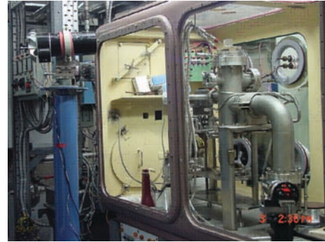
Figure 4: Spot technique for measurement of solidus-liquidus temperature of fuel materials
