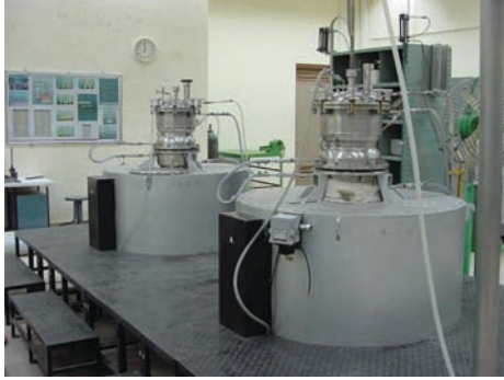
Figure 3: Pilot plant for elemental boron production
