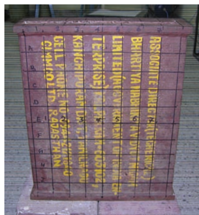
Fig. 5 Lead shots filled PI flask shell mockup
