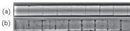
Fig. 5 Neutron radiographic image showing portion of (a) Unirradiated and (b) Irradiated MOX fuel pin
