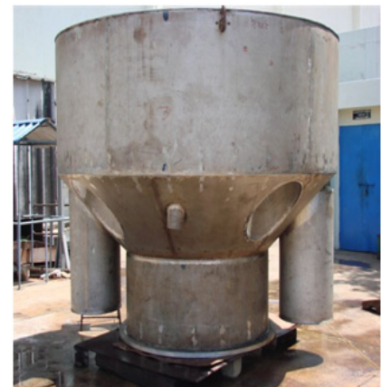
Fig. 1 PFBR inner vessel 1/4 th scale model
