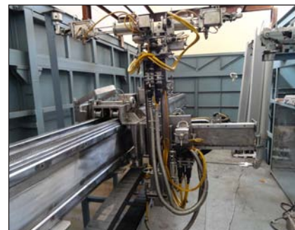
Fig. 2 Photograph of sample handling robot installed in mock-up facility
