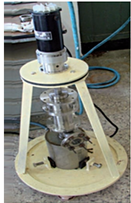
Fig. 1 Test setup for 25 mm diameter shaft
