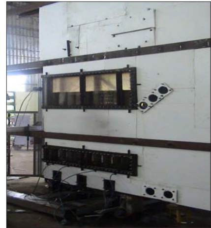
Fig. 2 Experimental slab model for inter wrapper flow studies
