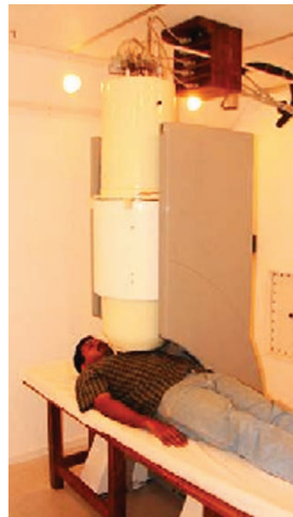
Fig. 1 37 channel cryostat positioned over the chest of a subject for Magnetocardiography
