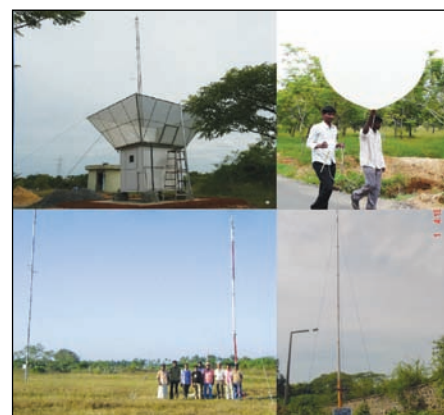
Fig. 1 Observational system at Kalpakkam with Met Towers, Wind Profiler, GPS radiosonde
