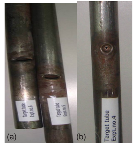
Fig. 2 Wastage on target tube in sodium at (a) 773 K and (b) 703 K
