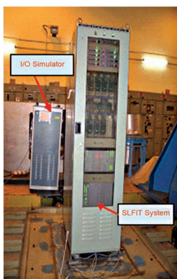
Fig. 2 SLFIT system on shake table
