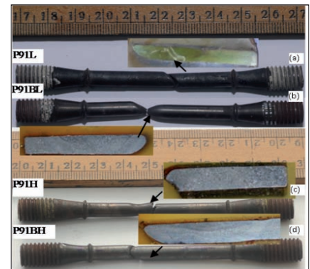
Fig. 4 Cross weld specimens creep tested at 873 K and 120 MPa
