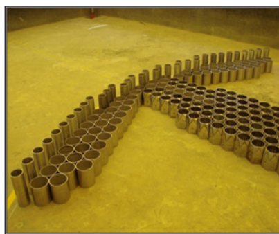
Fig. 1 Experimental setup with simulated core configuration of mock up subassemblies heads in the 10 m water tank
