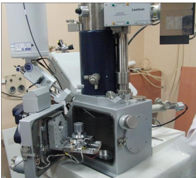
Fig. 2 Specimen being loaded in the SEM
