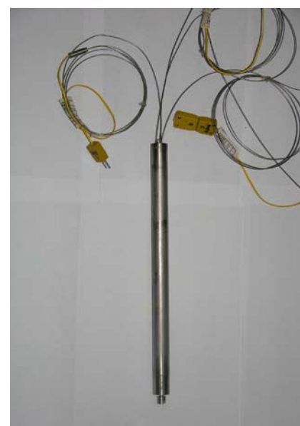
Fig. 2 Fabricated capsule with attachment of thermocouples
