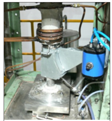
Fig. 3 Crucible with coil and valves
