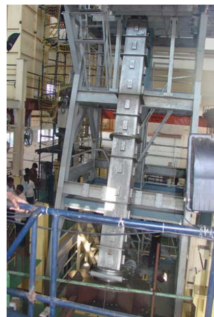
Fig. 1 Primary ramp and tilting mechanism test assembly
