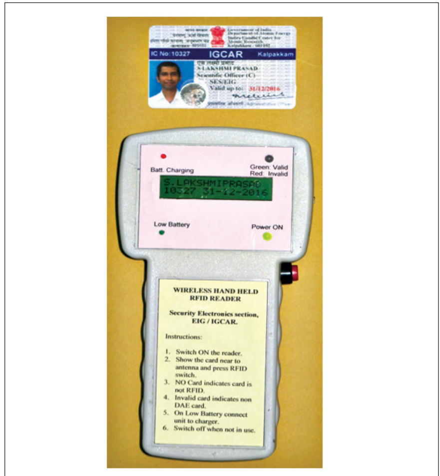
Fig. 1 Hand held RFID reader
