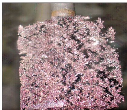
Fig. 1 Uranium metal deposit on solid cathode covered with salt
