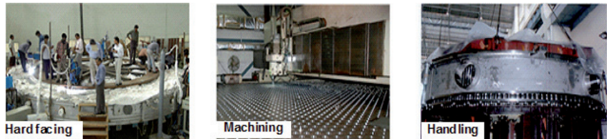
Fig.1 Manufacturing stages of grid plate
