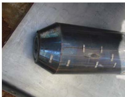
Fig. 3 Electromagnet with thermocouples fixed on it
