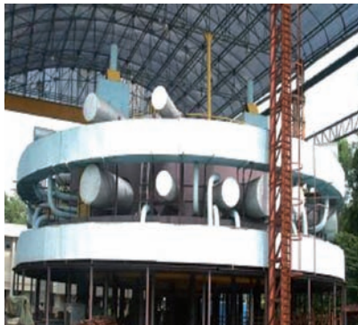
Fig. 5 Full scale top shield layout mockup
