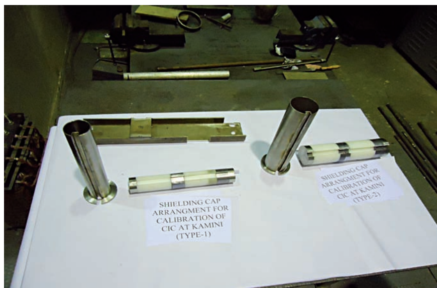
Fig. 1 Shield plug for detector testing
