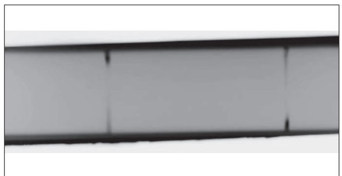
Fig. 3 Neutron radiograph showing the nickel blocks inside the subassembly
