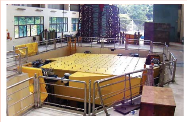
Fig. 1 High capacity seismic shake table
