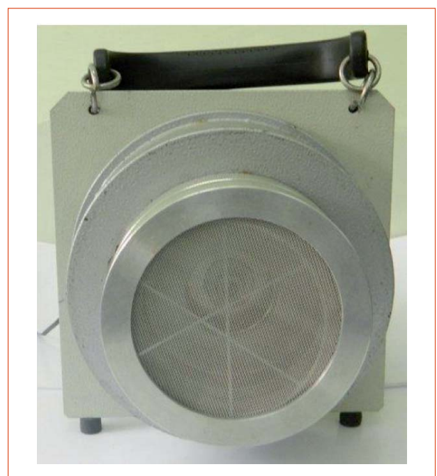
Fig. 1 Photo of indigenously developed air sampler
