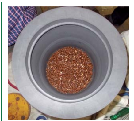
Fig. 2 Copper pellets before melting
