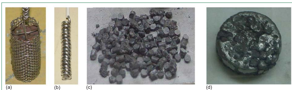
Fig. 2 (a) UO_2 pellet feed (100g) (b) platinum coil anode (c) processed pellets and (d) consolidated uranium metal
