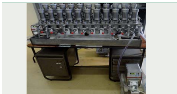
Fig. 1 A view of experimental setup for testing DFRP centrifugal extractor banks
