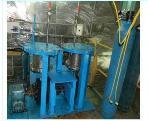
Fig. 3 Actuator mechanism with bellows
