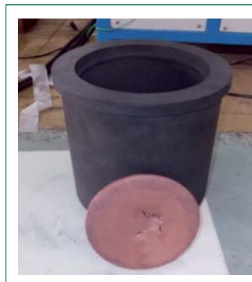
Fig. 4 Copper ingot after melting
