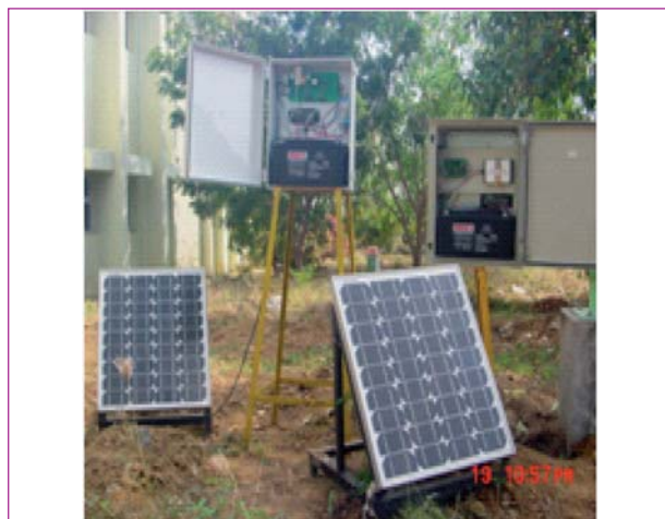
Fig. 1 Autonomous gamma dose loggers and argon fluence monitor in the field
