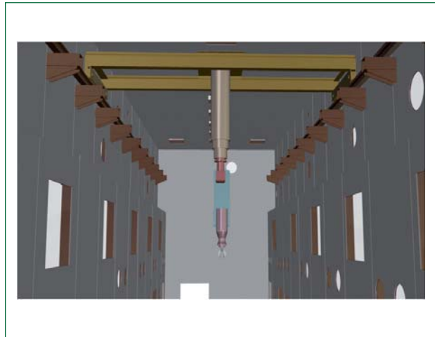
Fig. 1 3D model of power manipulator inside containment box
