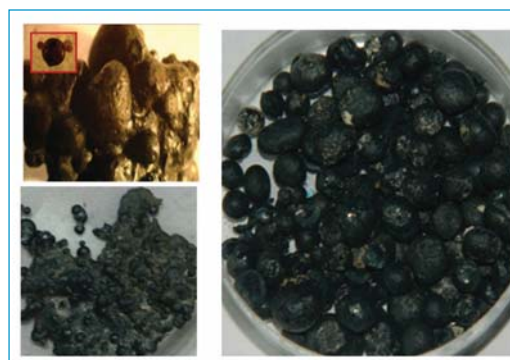
Fig. 4 Typical debris from high temperature ceramic simulant
