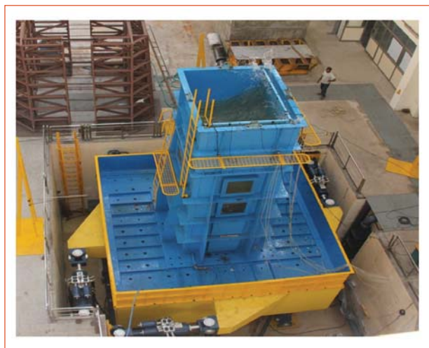
Fig. 4 Seismic testing of spent fuel trays
