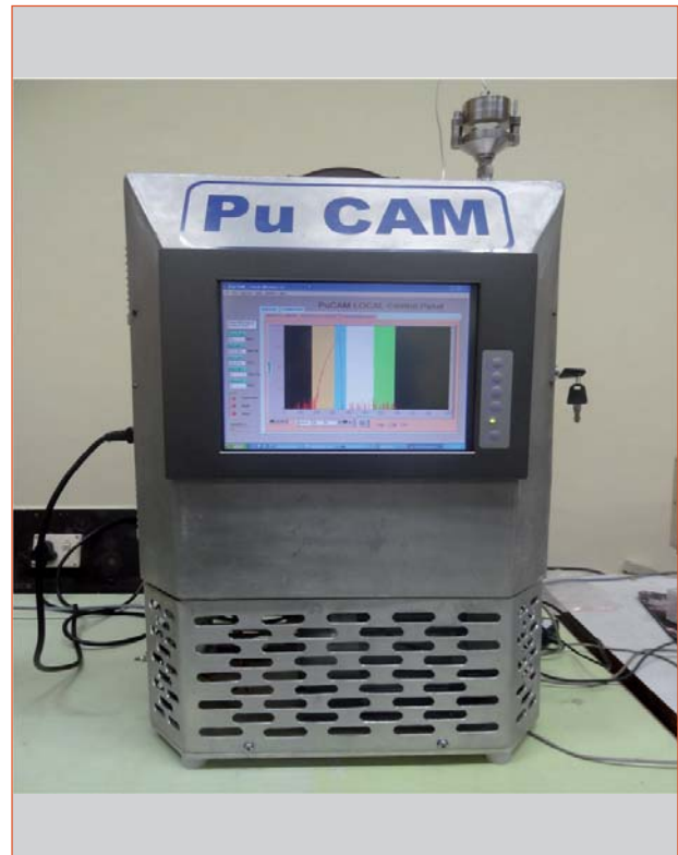
Fig. 1 Indigenous plutonium continuous air monitors
