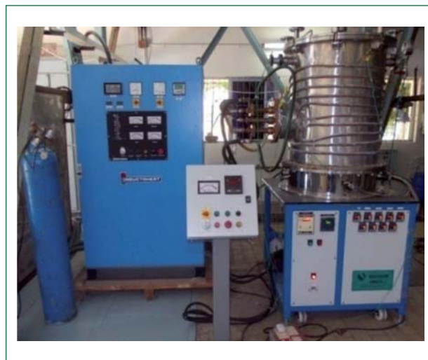
Fig. 1 Induction heating system
