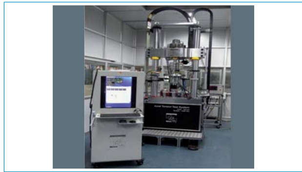
Fig. 4 Axial torsion testing system at metal forming and tribology programme
