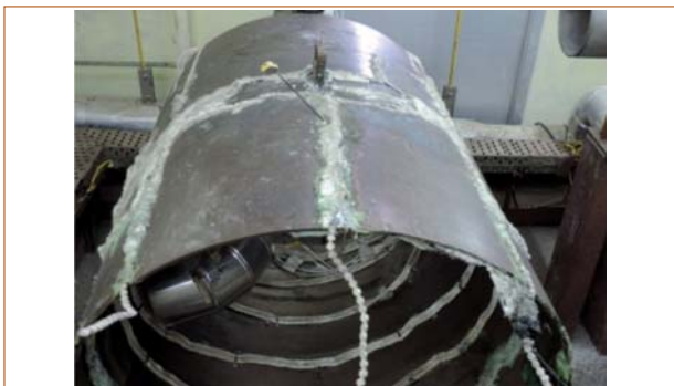
Fig. 1 Test section 1 after sodium leak experiment
