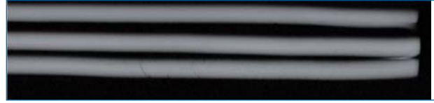
Fig. 3 X-radiograph of U-6Zr slugs
