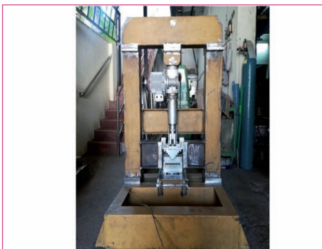
Fig. 1 RSA & FSA fuel pin chopping assembly
