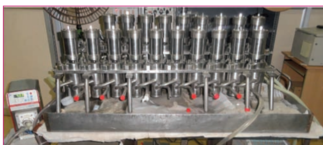
Fig. 1 20-Stage CE 40 mm bowl with inter-stage pump
