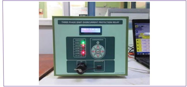
Fig. 3 Fabricated Numerical Over-current Relay Unit
