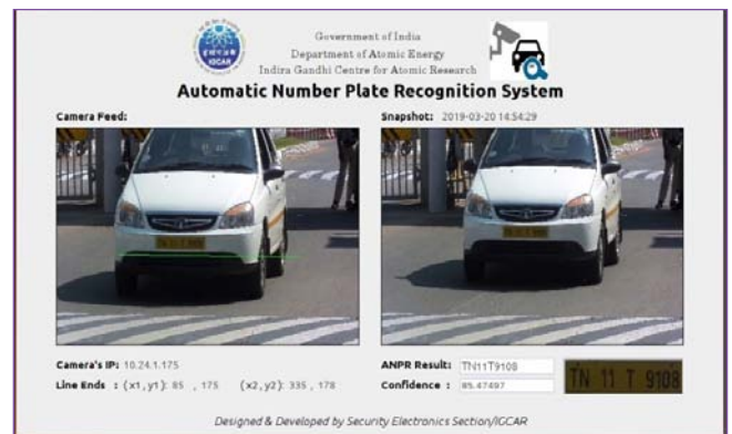
Fig. 1 Capturing the registration number of the vehicle with image of the number plate using video analytics and automatic recognition system
