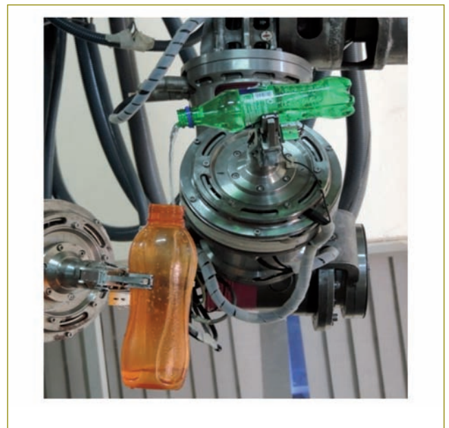
Fig. 6 Delicate operations using servo manipulator
