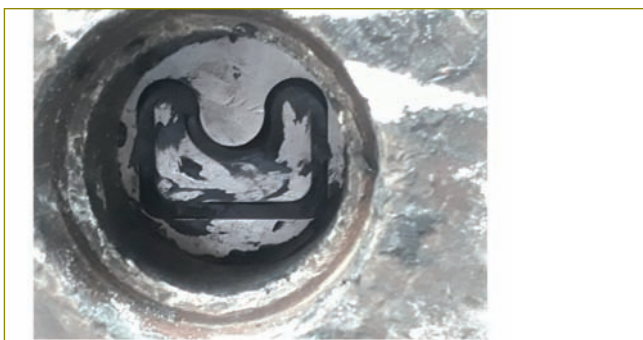
Fig. 1 Inflatable seal being extruded
