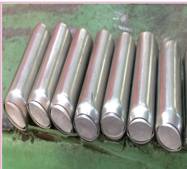
Fig. 4 Chopped pieces of RSA dummy fuel pins
