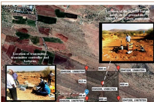
Fig. 1 Photograph of the experimental site along with the coordinates of the 400 m x 400 m transmitter loop and the experimental setup.
