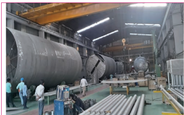
Fig. 1 Fabrication of shells
