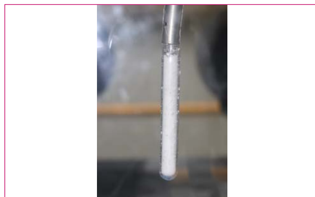
Fig. 3 Salt sample after chlorination
