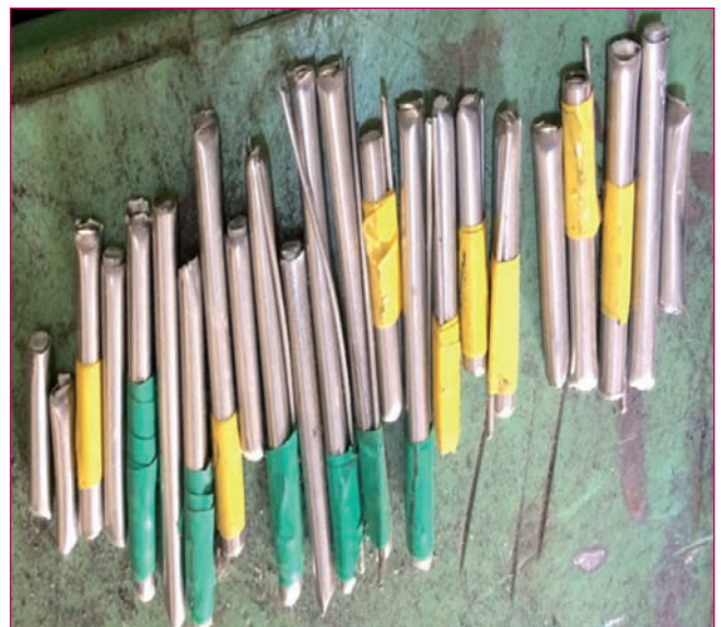
Fig. 5 Chopped pieces of FSA dummy fuel pins
