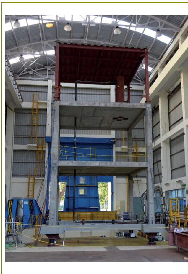
Fig. 1 Base isolated Multi storey building with equipment and piping on shake table
