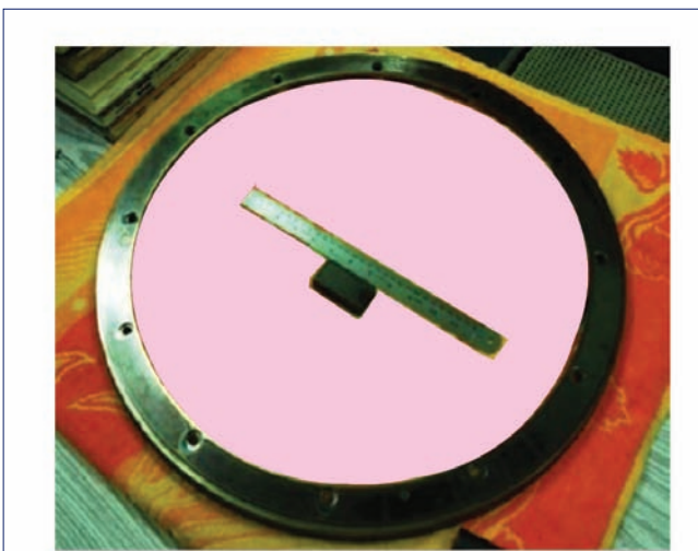
Fig. 1 Plasma nitrided casing ring and test specimen
