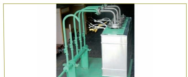
Fig. 3 Setup for Sodium compatibility testing
