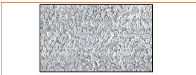
Fig. 1 Micrograph of Al 0.97 Ga 0.03 N nanorods
