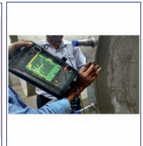
Fig. 3 UT of Corner weld
