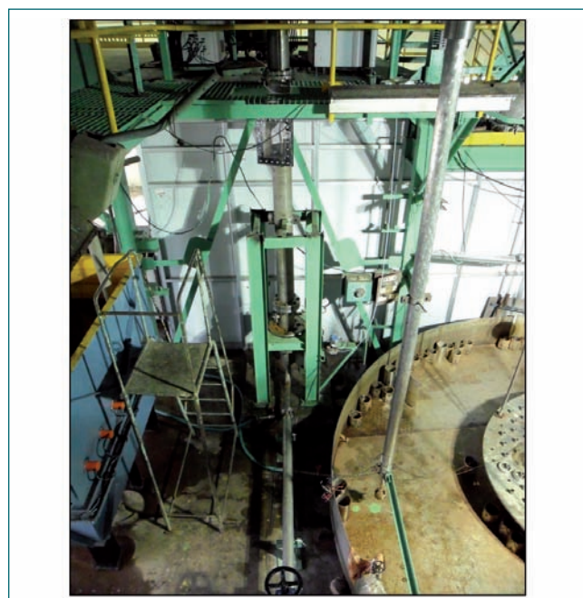
Fig. 3 View of water loop test section at Hall II for pressure drop and lifting force studies
