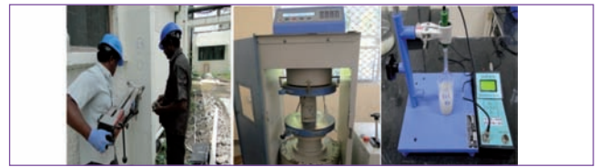
Fig. 2 Semi destructive coring and laboratory assessment
