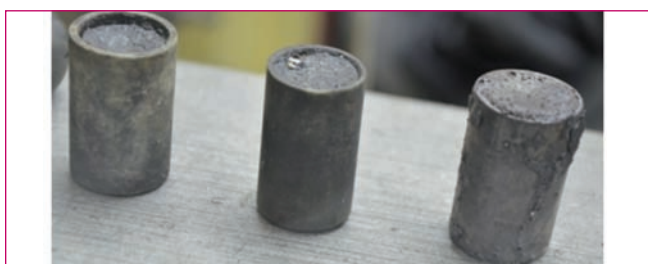
Fig. 1 Typical liquid Cd cathodes used for molten salt electrorefining of U-Pu-Zr alloy
