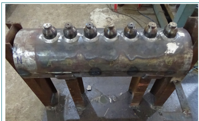
Fig. 1 Welded thermal baffles on header
