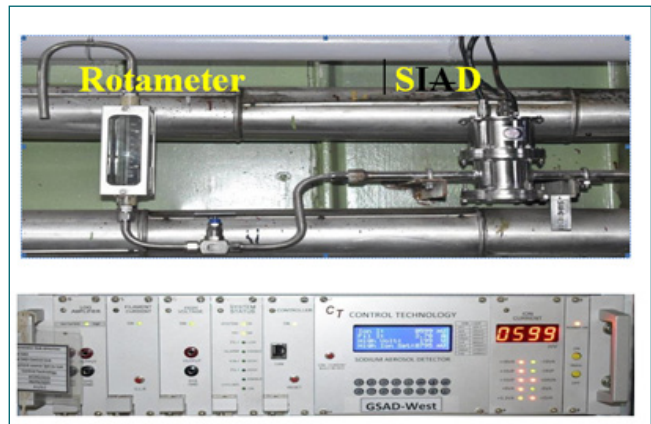
Fig. 2 Sensor and electronics of Global GSLDS
