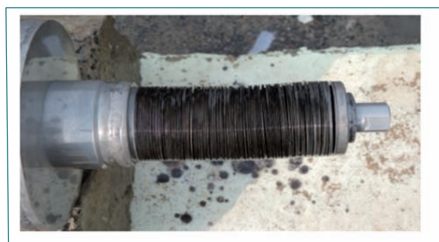
Fig. 3 Gripper bellows after sodium cleaning
