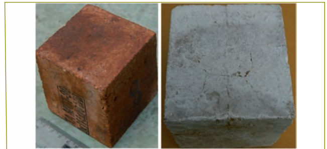
Fig. 2 MgO bricks before and after thermal shock testing
