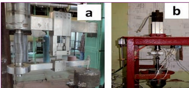
Fig. 5 (a) Setup for qualification of improved guide & rail using robust transfer arm gripper at LCTR and (b) Setup for qualification of geometry modification of actuator rod
