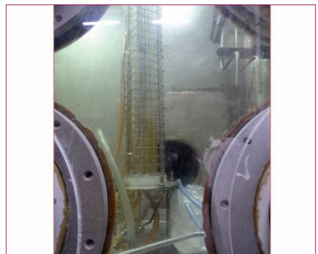
Fig. 3 Plutonium oxalate precipitation in PuRC
