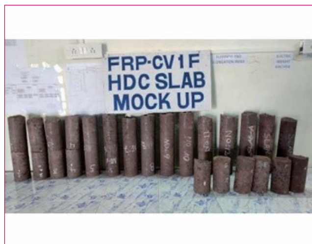
Fig. 2 Core samples drawn from mockup slab
