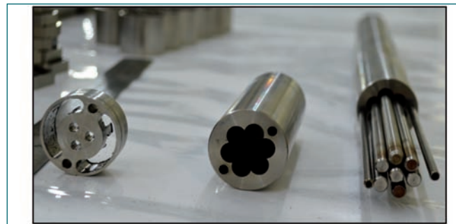
Fig. 2 View of end plugs, intermediate plugs, and arrangement of dummy pins in the capsule
