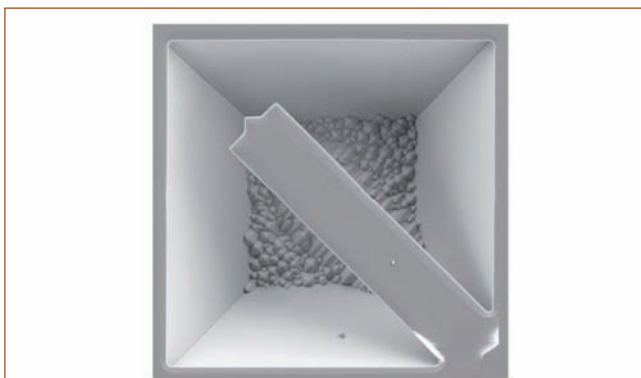
Fig. 1 FESEM image of a typical SiO 2 MC fabricated using DLW and wet chemical etching methods
