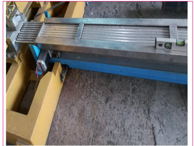
Fig. 3 Magazine assembly with chopper
