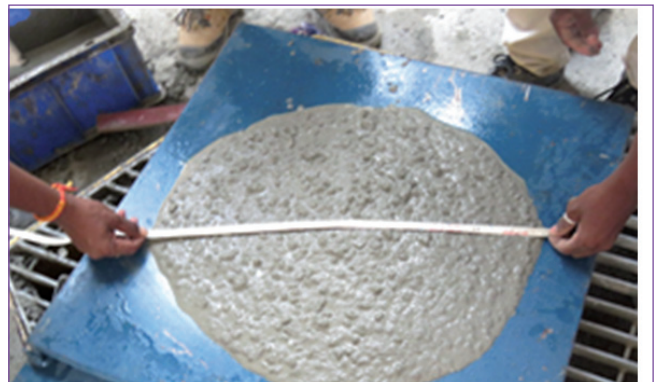
Fig. 2 Flow-ability using slump flow test
