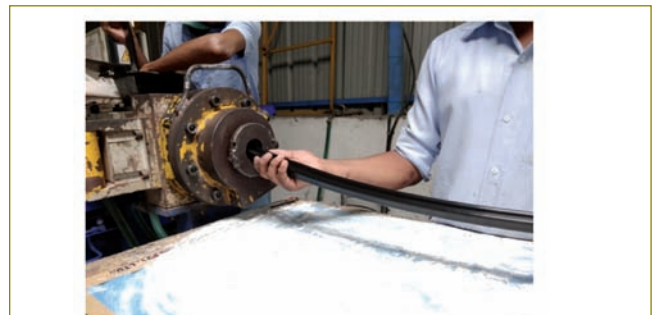
Fig. 2 Seal being extruded
