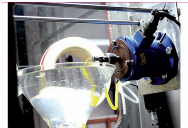
Fig. 2 Feed tank and vibrator positioning
