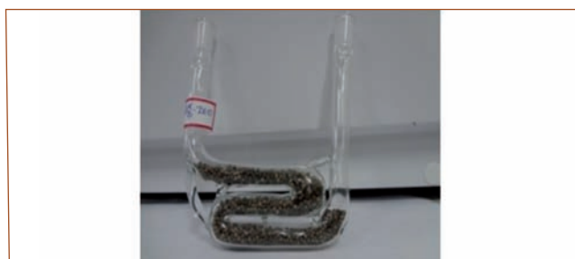
Fig. 2 Modified tube with Zeolite
