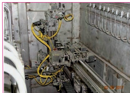
Fig. 6 Sampling handling robot inside cell
