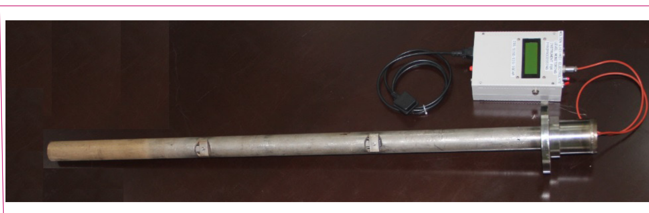
Fig. 2 Level Probe of 1 meter range with instrument
