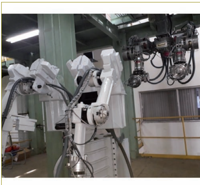
Fig. 5 Photograph of servo manipulator for hot cell applications
