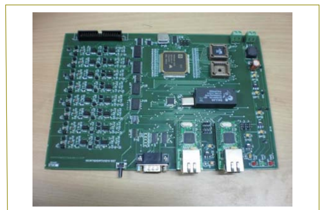
Fig. 3 Fabricated PCB of remote data acquisition system
