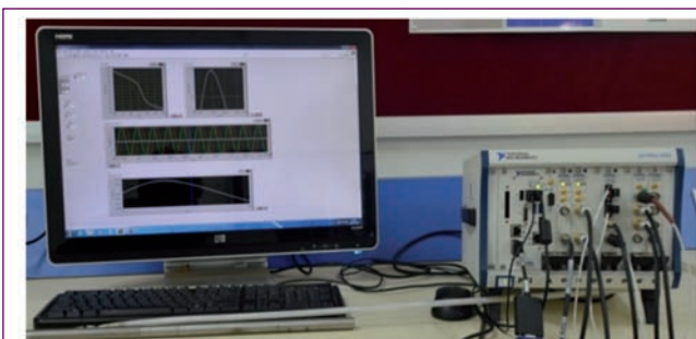
Fig. 1 Photograph of the in-house developed SFRFEC instrument with LabVIEW control software
