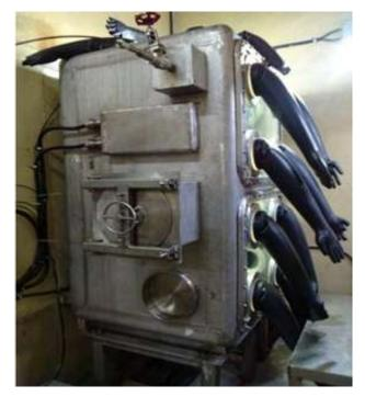
Fig. 2: View of incell crane drive glove box
