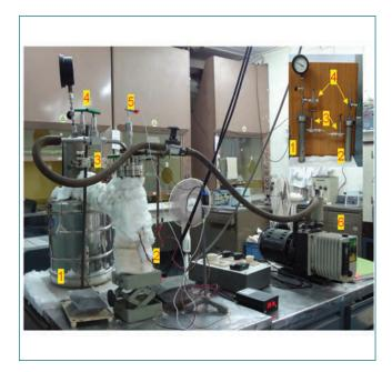
Fig. 3 photograph of the experimental setup used for cleaning sodium by vacuum distillation. (1) distillation vessel kept in a furnace, (2) sodium collection vessel with insulatin, (3) SS below sealed valves for sodium, (4) bellow sealed valves for argon gas, (5) level probe, and (6) rotary vacuum pump
