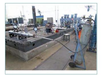
Fig. 13 Pneumatic testing of ALIP
