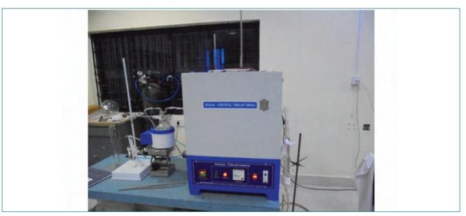
Fig. 1 Pyrohydrolysis facility for boron recovery
