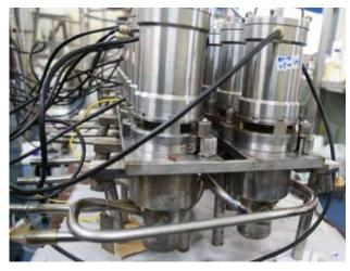
*Fig.2:* View of the modified inter-stage organic and aqueous pipe lines connected in-between 10<sup>th</sup> (Right) and 11<sup>th</sup> (Left) stages
