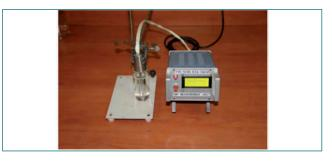
Fig. 1 Photograph of the embedded unit along with the capacitive type probe
