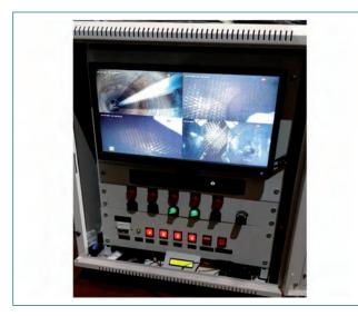
Fig. 4 RCVS control panel with images
