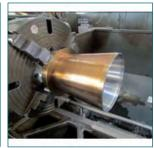
Fig. 6 Vertical honing of outer duct
