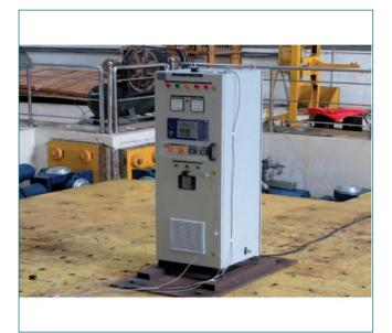
Fig. 1 Prototype 48 V DC charger in shake table
