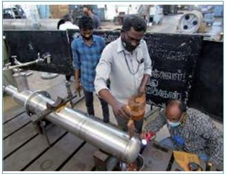
Fig. 14 Quality checks after pneumatic testing
