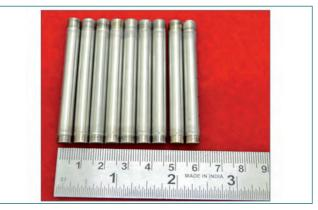
Fig. 3 Fabricated pressurized capsules of IFAC-1 SS (clad tube) & SS 316LN (plug) using laser welding and ready for biaxial creep tests
