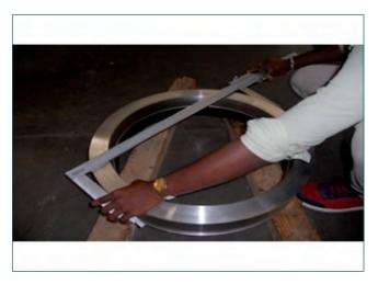
Fig. 2 Outer diameter measurement
