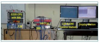
Fig. 2 Test setup in Lab
