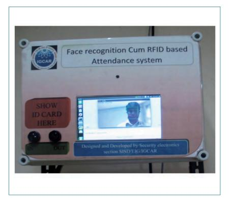
Fig. 1 Face recognition in Security Electronics Section
