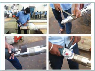
Fig. 1 Photos show radius is being formed in DSA adopting traditional method using filing and hand Grinding techniques
