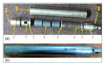
Fig. 2 Photographs of (a) components used for making absorber pin [1. D9 clad, 2. bottom plug, 3. top plug, 4. B<sub>4</sub>C pellets, 5. support disc, 6. spring, 7. support sleeve, 8. sodium entry and 9. sodium exit] and (b) assembled view
