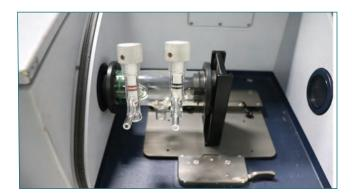
Fig. 2 CO<sub>2</sub> gas sampler placed inside the sample compartment of IR spectrometer
