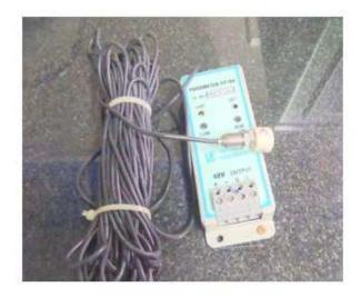
Fig.2: Sensor with pre-amplifier
