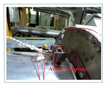
Fig. 2 Photograph of sensor locations at dish end on ALIP
