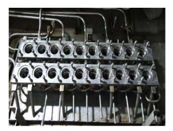
*Fig.4:* Photographic view of modified 20 stages larger dia ACE stationary bank inside the DFRP cell
