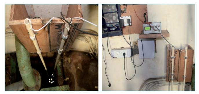
Fig. 1 WQMS consisting of conductivity probe, temperature probe installed at RCL site
