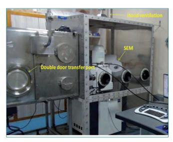
Fig. 1 SEM with glove box interface
