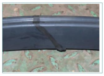
Fig. 2 Test seal with in-situ joint
