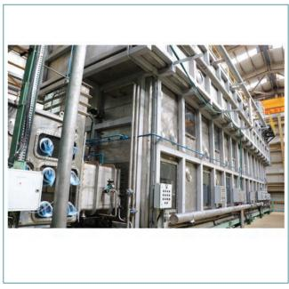
Fig. 1 PPRDF 500m<sup>3</sup> containment box
