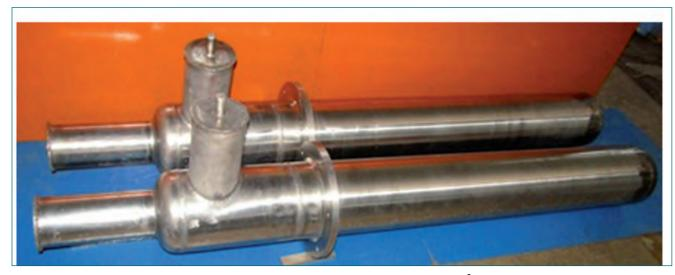
Fig. 15 Inner and outer duct assemblies of PFBR annular linear induction pumps of 170 m<sup>3</sup>/h capacity
