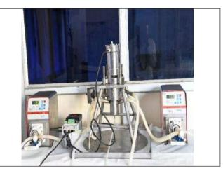
Fig.2: Experimental setup for chocking of centrifugal contactor bowl
