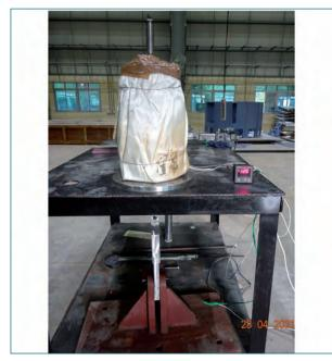
Fig. 3 Photograph of CSRDM gripper screw test setup
