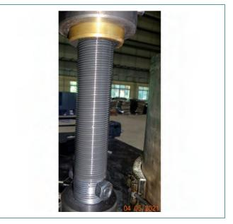
Fig. 4 Grease lubricated mock-up gripper operating tube (screw) after testing
