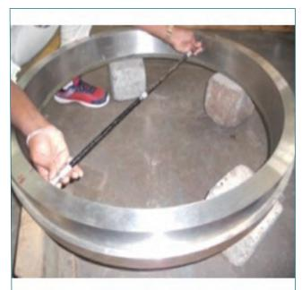
Fig. 3 Inner diameter measurement
