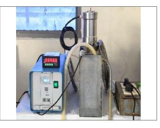
Fig.1: Equipment for ultrasonic cleaning of centrifugal contactor bowl
