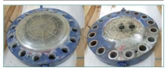
Fig. 1 Photograph of top flange of diaphragm compressor
