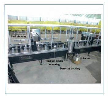
Fig. 1 Gamma scanning system
