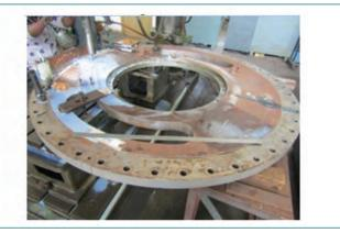
Fig. 8 Ratchet support flange machining in Radial Drilling Machine
