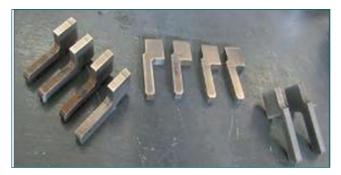
Fig. 9 Hardfaced spacers
