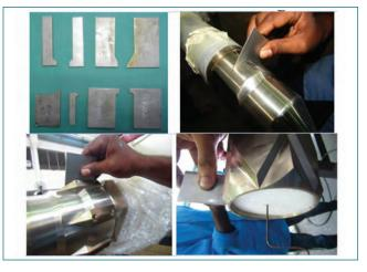
Fig. 3 Photos show machined gauges and their usage on the DSAs
