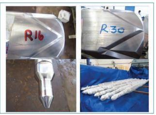
Fig. 2 Photos show radius formed DFSA ends, Discriminator guide portion and completed DFSAs
