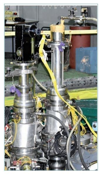
Fig. 1 Periscope and projector as installed in the pile
