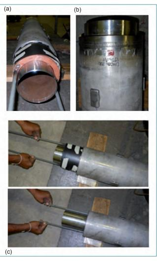
Fig. 4 Sequence of operation (a) Placement of film on the tool (b) Marking and IQI placement (c) Insertion of film cassette inside the annular gap
