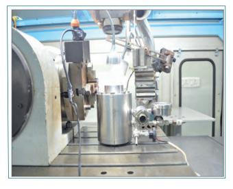
Fig. 2 LASER welding setup for sealing of pressurized capsule inside the pressure chamber
